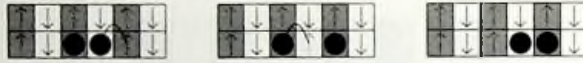
Figure 8.14: Two holes can move together without creating an intermediate double occupied state. Therefore, holes want to form real-space pairs. A hole pair can move if a single electron makes two hops.
